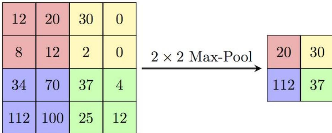
**Figure 3: Representation of Max-Pooling Layer [21]**
